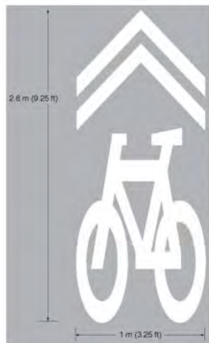
Typical Pavement Marking on Designated Shared Road
